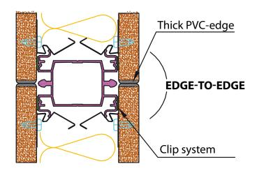
You can combine different styles to get different effects: for example, using the « edgeto-edge » system on one side will give your partition real class, while the use of joint-covers will give a more classical effect.
