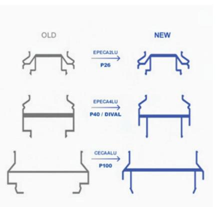
Improved clipping, ease of assembling / disassembling and durability are the main advantages of the new spacers.
